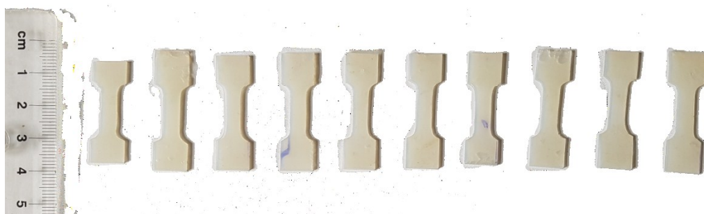
Fig. 5.2 Samples of virgin homogeneous material made from Laripur LPR 5020 high density polyurethane (HDPU).
