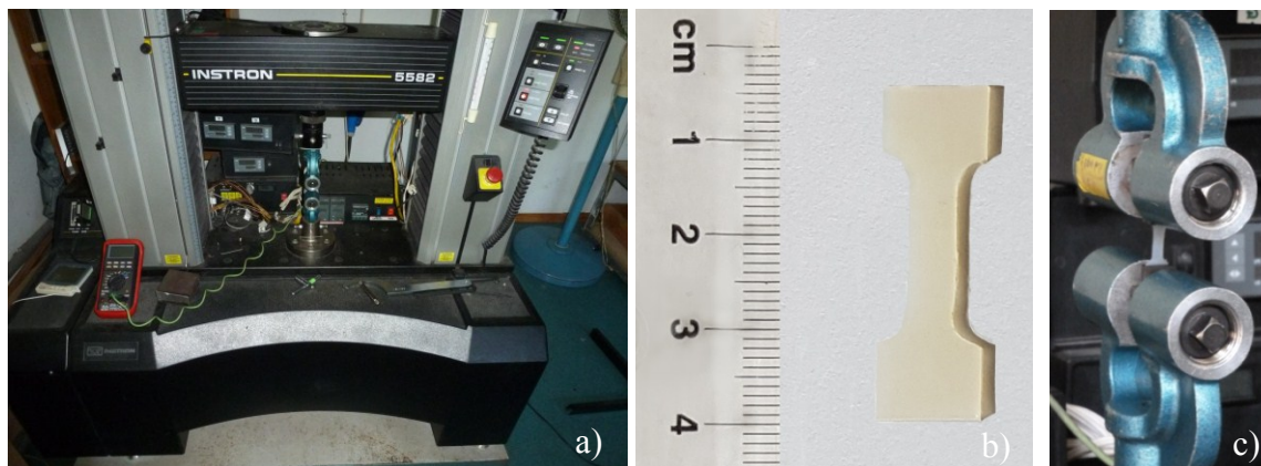
Fig. 5.1 Test bench (a) test specimens (b) and zoom on the test specimen (c) used for uniaxial stretch of high density polyurethane Laripur LPR 5020.
