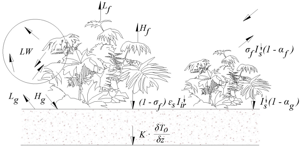
Figure 8.5. Simplified representation of the energy balance in the passive construction (source: on the basis of Sailor, 2008, Kumar, 2017).
